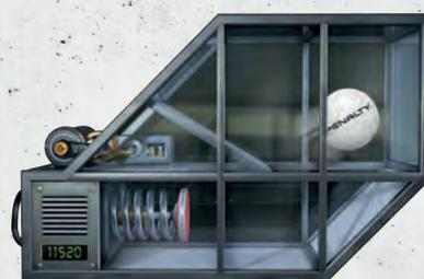
A BOLA É ATIRADA 7 MIL VEZES CONTRA UMA PLACA DE AÇO A 50 KM/H. AS COSTURAS, A VÁLVULA DE AR E AS CARACTERÍSTICAS DA BOLA DEVEM PERMANECER INTACTAS.
